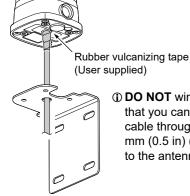
(i) DO NOT wind the tape too thick so that you can later thread the coaxial cable through the bracket hole (12 mm (0.5 in) (d)) to attach the bracket to the antenna.
