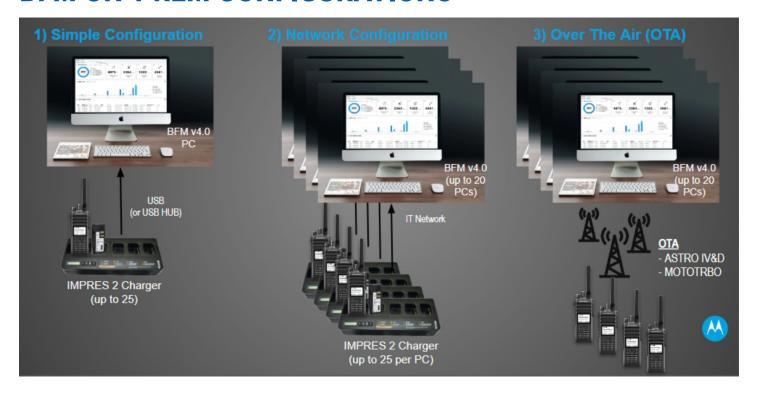
Motorola Solutions' Battery Fleet Management (BFM) V4.0 supports the following three (3) on-prem methods of gathering IMPRES battery data:
