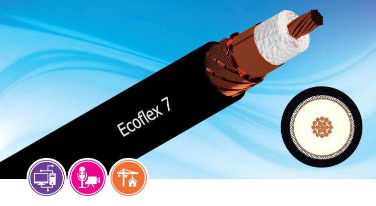
Ecoflex 7 is a highly flexible coaxial cable designed for the frequency range up to 6 GHz. The extremely low attenuation and small bending radius of this cable make it interesting and recommended for many applications in high-frequency technology.
