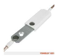
Small and flat grounding plate 20x80 mm for installation directly on top of shielding products and grounding straps. For the skirting board area. **Installation preferably in the baseboard area (due to its small grounding surface) with shielding paint, shielding mesh. Usage only on the interior.** One piece per wall is necessary due to the small contact area. Height when completely mounted is only 4 mm (without cover) or 6 mm (including cover).
