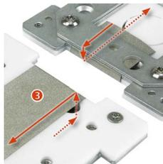
3 | Glue grounding strap/EMV strap or prepare stainless steel tape/stainless steel mesh for clamping. If the case should be mounted directly on a shielding product, clamp the grounding strap and glue it across the backside.
